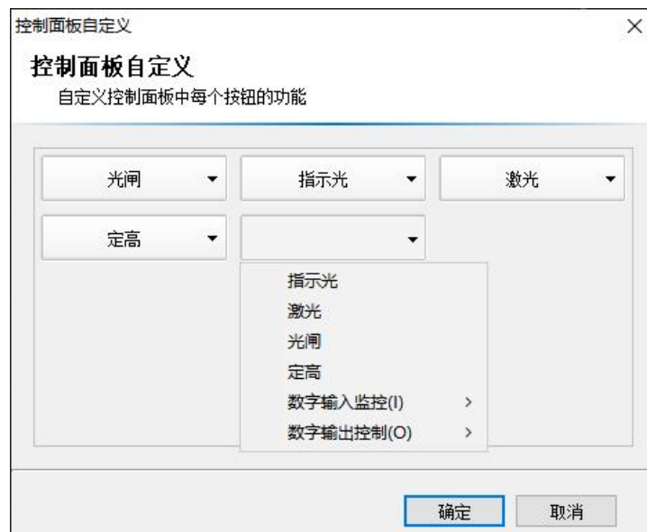
Figure 74 Control panel custom configuration
