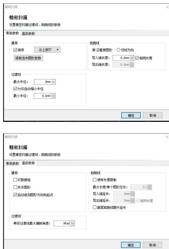
Figure 44 Array runway flying cut parameter setting
