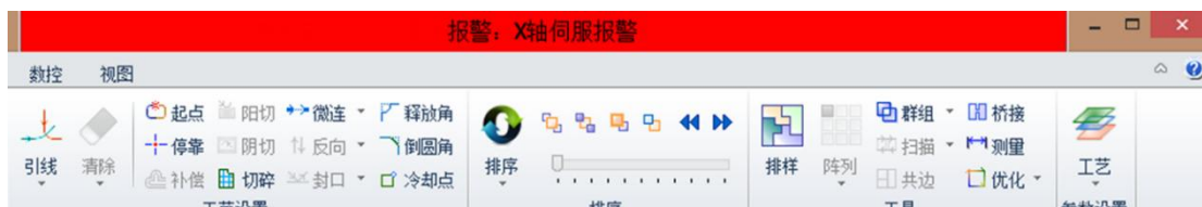
Figure 70 Alarm message indication
