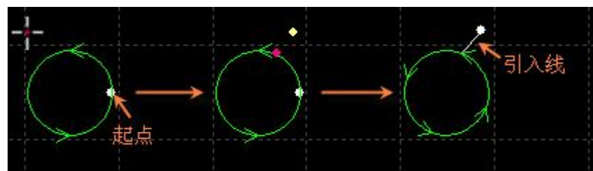
Figure 37 Manually add an incoming line
