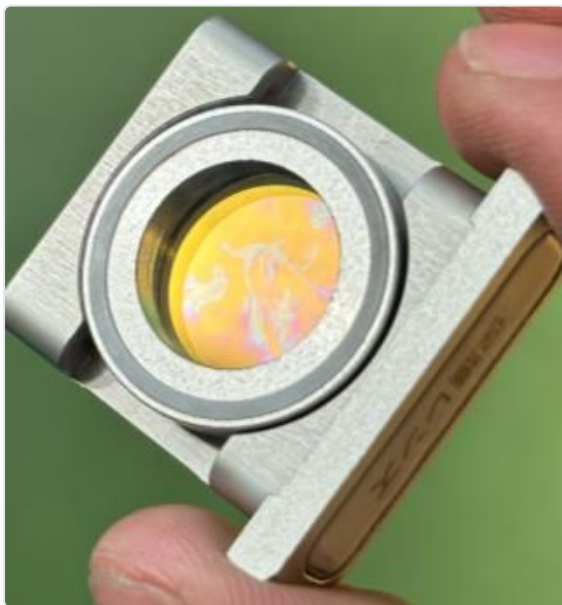
Figure captions: Photo of a fiber laser crystal section damaged by reflection / Photo of oil adhering to the protection lens
