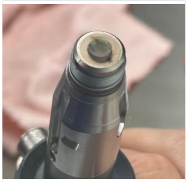
Figure captions: Photo of a fiber laser crystal section damaged by reflection / Photo of oil adhering to the protection lens
