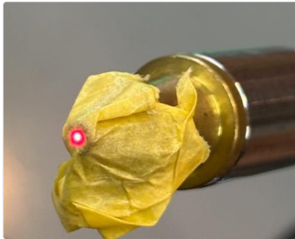
Figure captions: Beam path correctly aligned / Beam path misaligned
