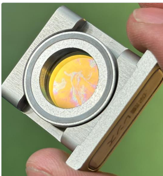
Photo: crystal section of the laser source destroyed by reflected laser / Photo: oil on the protection lens
